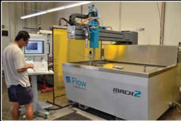
**Excellent Work Table Accessibility on a Machine Built for the Rigors of Waterjet Cutting**
